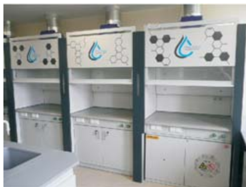
Fume hood with reduced height, to be installed in rooms with lower ceilings.
