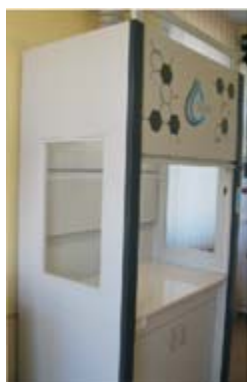
Fume hood with glazing on both sides
